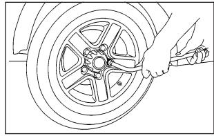
1. If your vehicle has wheel nut caps, remove them by turning the wheel wrench counterclockwise.
